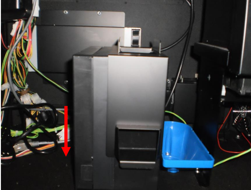
Figure 10: Coin Hopper Remove Direction
