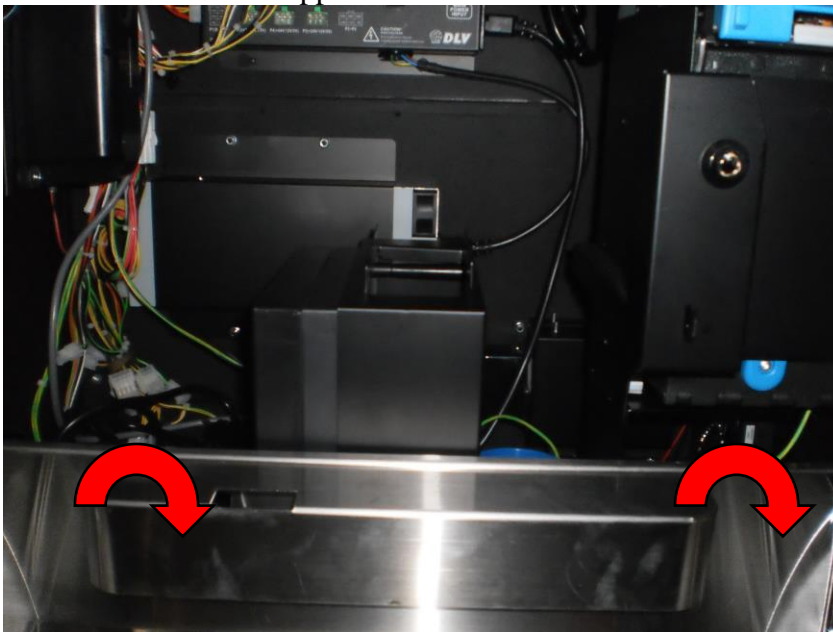
Figure 9: Coin Tray Remove Direction
